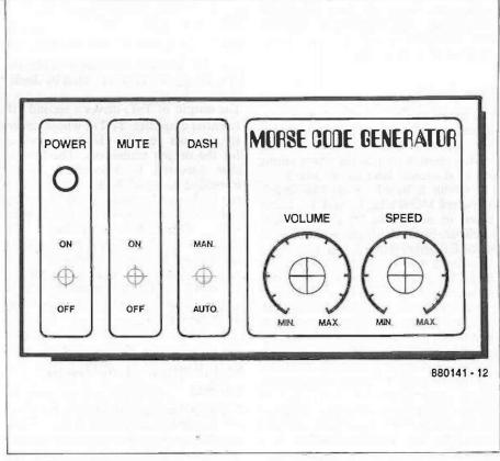
Fig. 2. Suggested front-panel layout.
