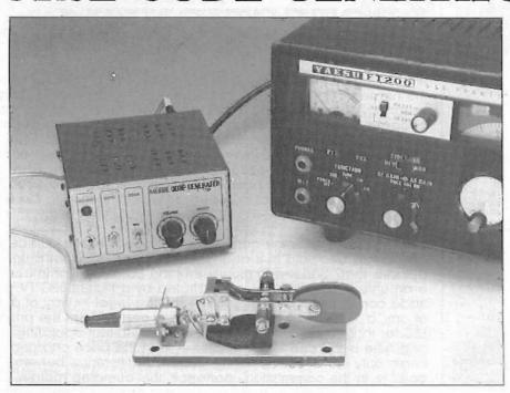
Ideal for both the morse trainee and the experienced operator, this low-cost, versatile, generator with relay output provides automatic timing, at a user-defined speed, of audible dots and dashes.
